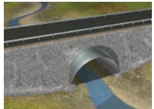
Then the road surface is completed with safety barriers.
