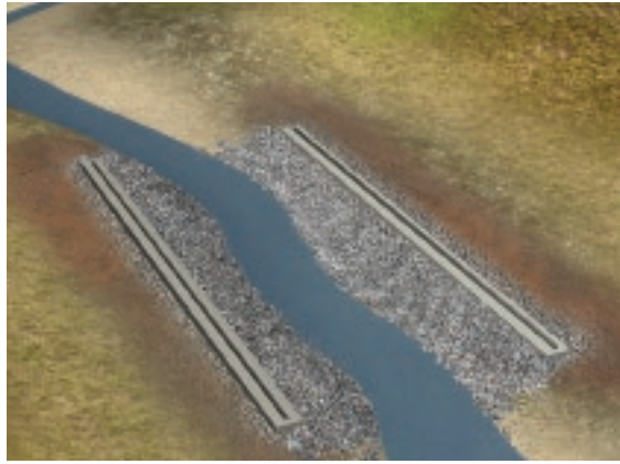
Reinforced concrete footings are cast over the prepared site.
