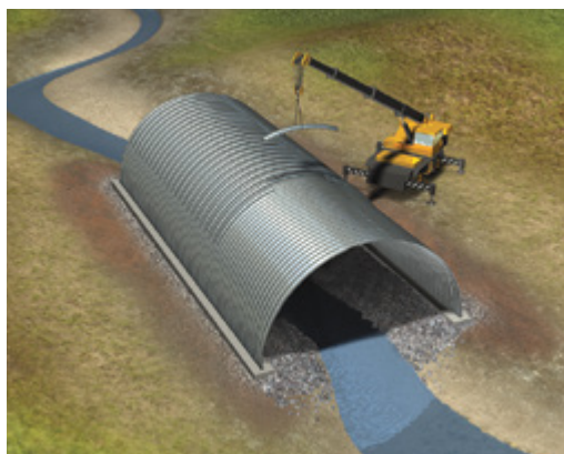
If specified, reinforcement ribs are then added.
